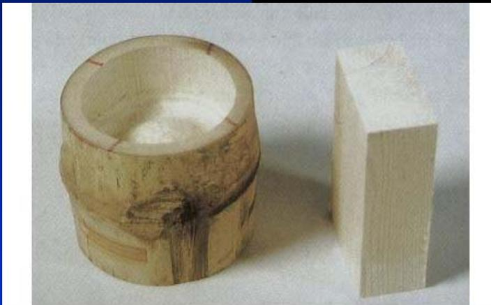
Fig. 42: Bamboo and timber pieces with the same area of cross-section
